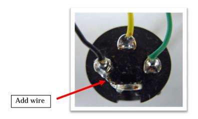
Add a short wire between the solder pad labeled "1" and the backplane ground solder pad.
